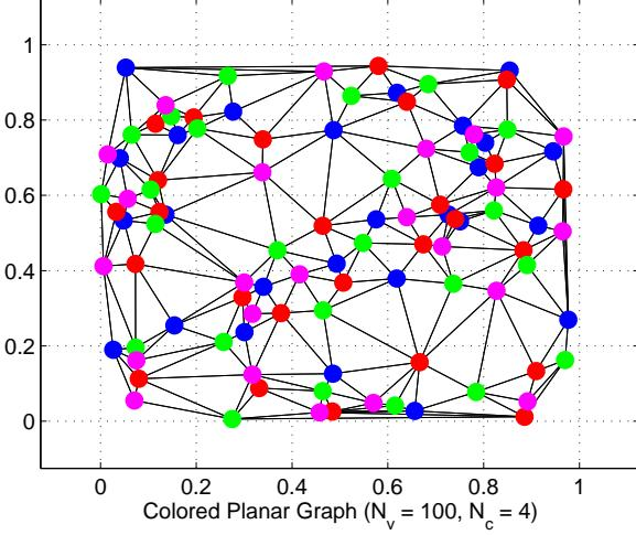
Figure 1: A planar graph with  $N_v = 100$  vertices that represent small cells, colored with  $N_c = 4$  colors, that can be regarded as orthogonal resources assigned to the cells in a non-conflicting way.
