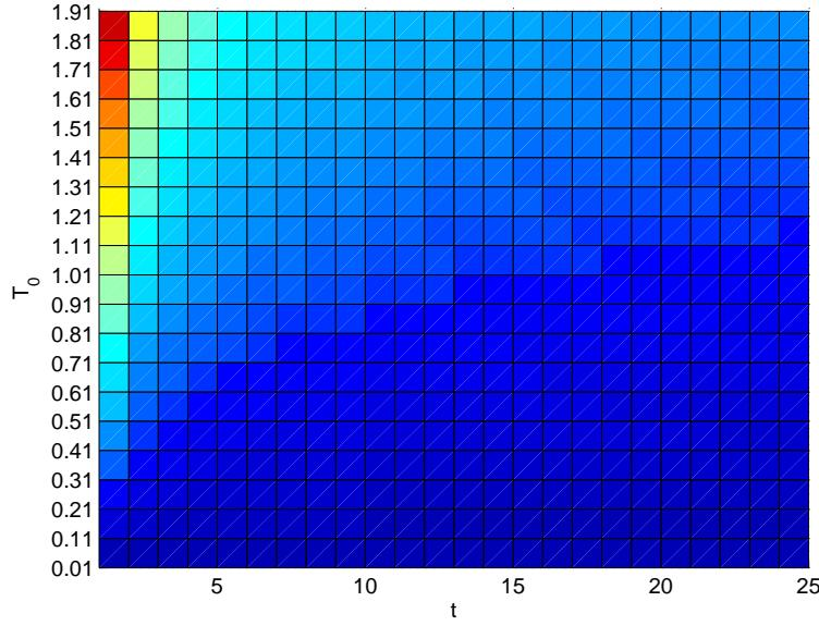
Figure 2: SA involves gradual reduction of temperature according to the cooling schedule  $T = \frac{T_0}{\log_2(2+t)}$  shown here, where  $t$  is the iteration index and  $T_0$  is the initial temperature.
