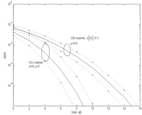
Fig. 3. Bounds on the BER performance, BPSK modulation format,  $N_T = 2$  and  $N_R = 2$ . Solid lines represent numerical BER estimates, dotted lines represent bounds (3), and single points report simulation results.
