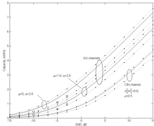
Fig. 2. Capacity per unit bandwidth,  $N_T = 2$  and  $N_R = 2$ . Solid lines represent numerical estimates of capacity, dotted lines represent bounds (3), and single points report simulation results. Squares represent estimates for low SNR (11).
