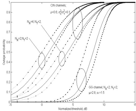
Fig. 1. Outage probability versus normalized threshold  $\gamma/\bar{\gamma}$ . Solid lines represent numerical estimates of outage probability, dotted lines represent bounds (3), and single points report simulation results.
