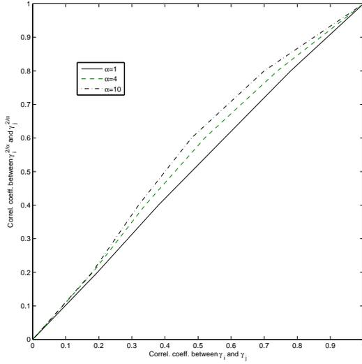
Fig. 1. Relations between  $R_{i,j}$  and  $\tilde{R}_{i,j}$  for  $\mu = 2$  and a few values of fading parameter  $\alpha$ .
