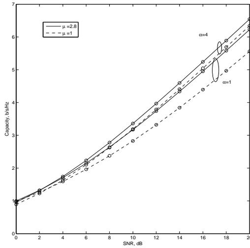
Fig. 2. Ergodic channel capacity per unit bandwidth (b/s/Hz), single-antenna transmission. Single points report simulation results.
