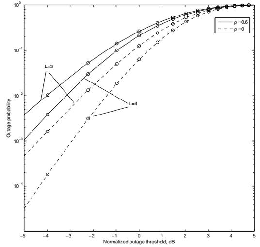
Fig. 4. Outage probability versus normalized outage threshold. Single points report simulation results.
