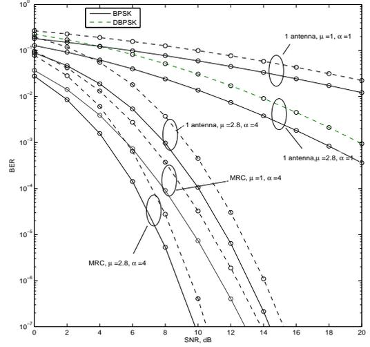
Fig. 3. Average BER for single-antenna transmission and for MRC over two independent branches. Single points report simulation results.
