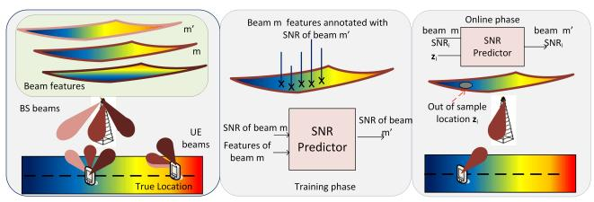
Fig. 3: Beam SNR prediction based on beam CSI feature: (Left); Construction of beam based features and their dimensionality reduction. (Middle); Beam feature annotation and SNR prediction (the offline phase). (Right); Beam SNR prediction based on beam feature (online phase).
