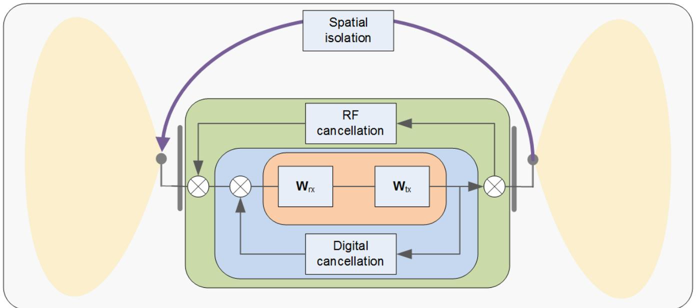
Figure 3. Self-interference cancellation mechanisms in a full-duplex relay.
