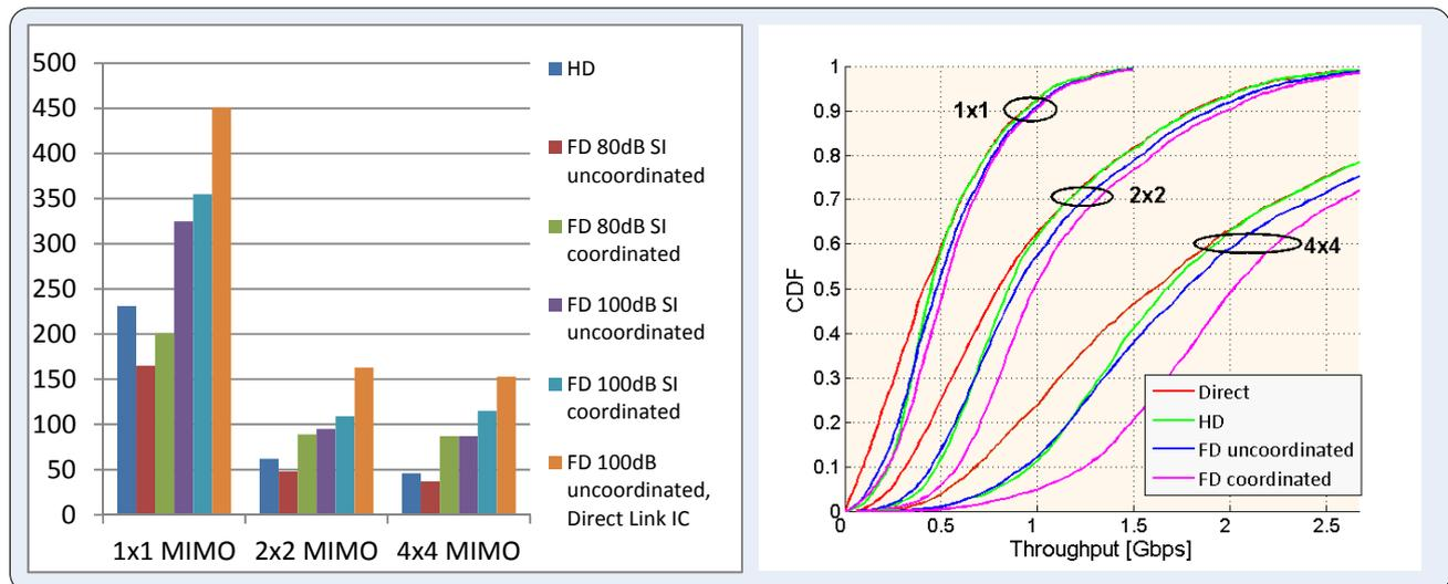
**Figure 4. MBB scenario: Left: Throughput at 5% of user throughput CDF, gain [%] relative to direct communication with F-AP only, i.e. (MultiHop- Direct)/Direct in %. Right: CDF of user throughput [Gbps], 1x1, 2x2 and 4x4 MIMO. Self-interference cancelation 80 dB at R-AP.**
