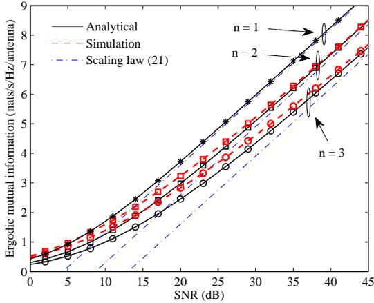
Fig. 3. Per antenna ergodic mutual information of multiple cluster scattering MIMO channels assuming  $K = 8$  with different numbers of clusters  $n - 1$ . In all cases, the number of antennas equals the number of scatterers per cluster. For  $n = 1$  the analytical curve is obtained from the exact ergodic mutual information formula derived in [17]. For  $n = 2, 3$  the analytical curves are obtained from the derived ergodic mutual information lower bound (14).
