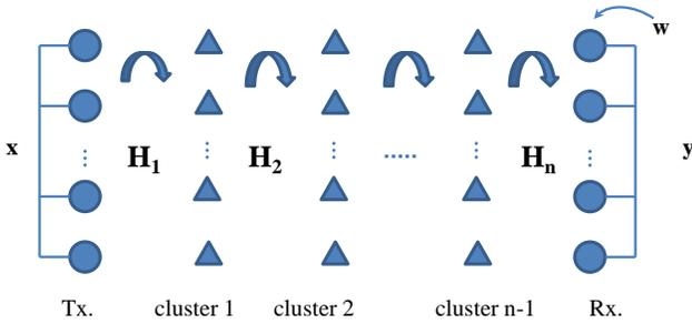
Fig. 1. Multiple cluster scattering MIMO channel with  $n - 1$  clusters. The number of antennas equals the number of scatterers per cluster.
